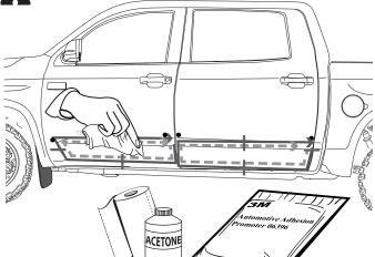
DRAW CENTER HASH MARK WITH GREASE PENCIL ON PANELS AND SHEET METAL, THIS WILL ENSURE PANELS WILL BE CENTERED TO GREASE PENCIL OUTLINE.
